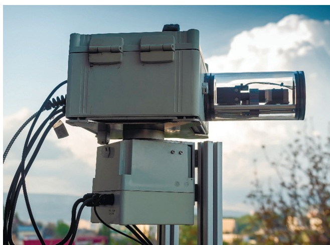
Urban measuring site: an autonomous meteorological complex for monitoring boundary layer parameters and a system for measuring the vertical distribution and total content of gas impurities and aerosols in the atmosphere..
